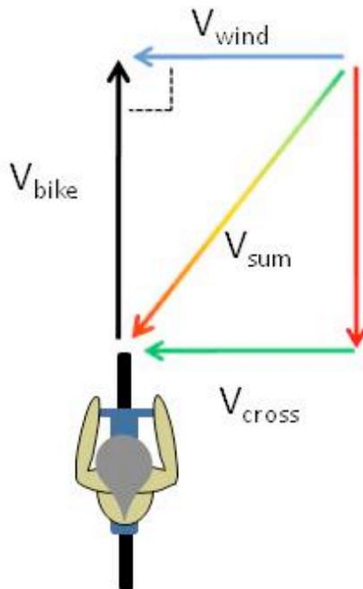
Figure 2. When wind comes in directly from the side, the crosswind is equal to the wind speed. The headwind speed is equal to the bike speed. But the perceived wind is greater than the two components, and it feels like it comes in from an angle.
