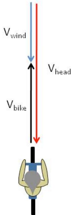
Figure 1. When the wind is directly against direction of travel, the total perceived wind velocity is the wind speed added to the bike speed.
