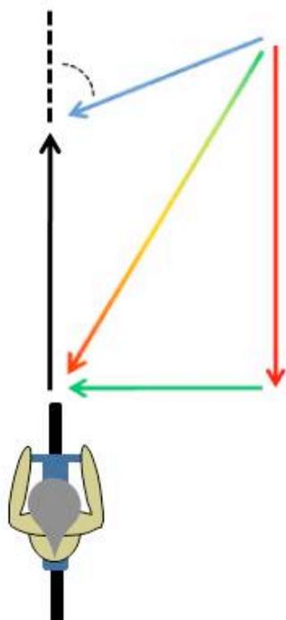
Figure 3. Wind coming in from different angles changes both the perceived wind velocity and direction.
