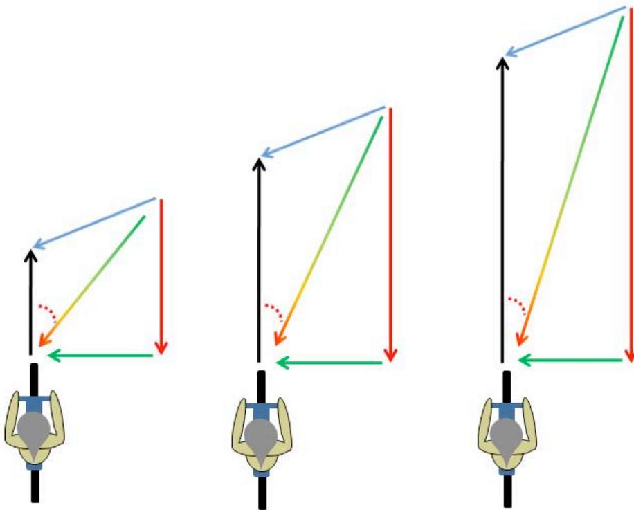
Figure 4. As rider speed increases, the headwind velocity component increases and the apparent yaw angle decreases.
